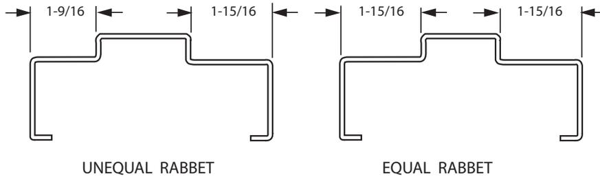
To ensure proper door operation with a standard templated hardware installed, **clearances** are designed into these frame dimensions.
