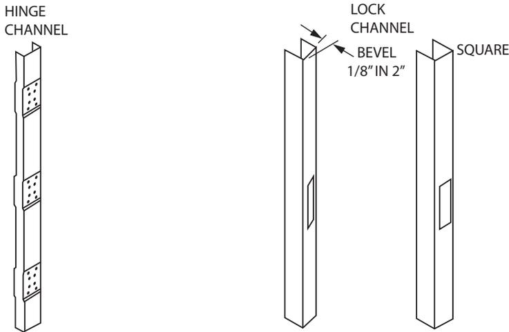
The **lock edge** of a CURRIES door is reinforced with a 14 gauge channel the full height of the door. A standard handed door lock channel is beveled 1/8" in 2" on the door edge. A standard non handed door lock channel is square on the lock edge. The non handed door lock edge is square to allow the use of it to be either right hand or left hand depending upon how the hinges are mounted on the hinge side.
