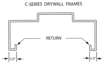
**NOTE:** Drywall frames are designed to fit snugly over the wall.
