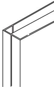
The “N” edge is a seamless door with additional welds, ground smooth then filled to conceal the seam.
