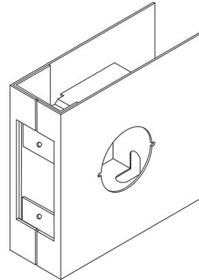
Lever handle locks requiring thru bolted trim holes can be factory prepared for ANSI A115.18 universal preparation using G2B code.
