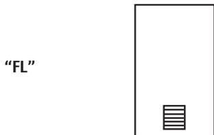
**FL** - Louvers are defined as an opening in the door face with a series of slats, blades, or piercings to allow passage of air. FL doors have a single louver located in the bottom of the door. CURRIES' standard louver is a fixed blade type that is rim mounted on the door face. Locations and sizes vary.
