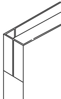
The “T” edge has the seam continuously welded the full height of the door, ground smooth and filled to conceal the weld.
