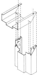
A strike jamb is typically mortised to receive a single lock strike plate. Other hardware preparations may include deadlock strikes, reinforcements for blanks or surface mounted strikes.
