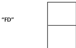
**FD** - Flush dutch doors are actually two separate doors. One occupies the bottom half of the frame opening and the other occupies the top half of the frame opening. Each operate independently and the bottom door can be furnished with a shelf.
