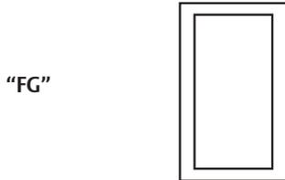
**FG** - Full glass lite doors are prepared to receive a glass lite covering the majority of the door face. Standard location is approximately 7-3/4" down from the top of the door, 6" in from the door edges, and 12" above the finish floor line on the bottom of the door.
