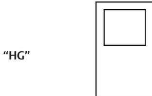
**HG** - Half glass lite doors are prepared for a lite that covers approximately the top half of the door. Standard sizes will vary with door size. Standard location is approximately 7-3/4" down from the top of the door to visible glass size and 6" in from the edge of the door to the visible glass size.
