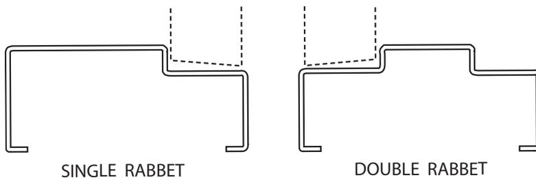
called “unequal” rabbet profile frames and are the most common. This allows the manufacturer to prepare for 1-3/4 inch or 1-3/8 inch doors on the same K.D. frame profile.
