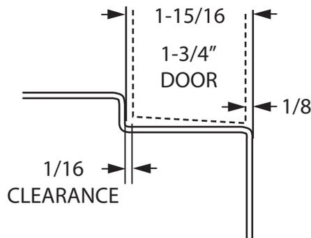
These clearances are fixed dimensions so all mortise hardware preparations are located on the doors and frames. Hardware preparation standards are recommendations established by A.N.S.I. (American National Standards Institute) "standards" for specific types of hardware (i.e., hinge, cylindrical locks, mortise locks, etc.).
