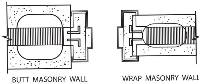
An existing wall construction (precast concrete) is another place for using the M series frame. This installation has the wall opening in existence and the frame butts to the wall and is bolted into place with anchor bolts.
