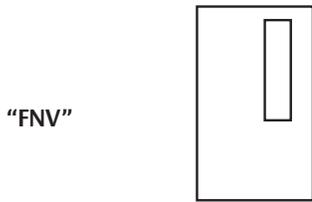
**FNV** - Narrow vision lite doors are prepared for long narrow lites of varying visible glass sizes and are located on the lock edge side of the door, approximately 6" in from the lock edge. CURRIES offers 10 standard size narrow lites.
