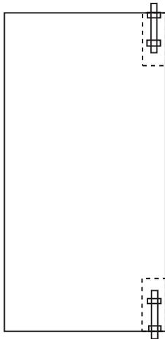
**NOTE:** Reinforcing channels are mounted top and bottom for surface application on the face of the door for these manual "slide" bolts.
