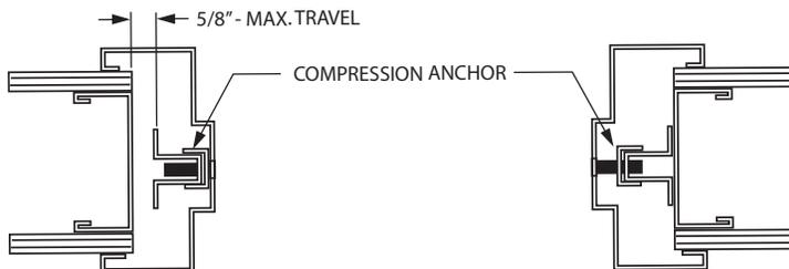
When the compression anchors are contacting the wall a preliminary squaring of the frame is done before the bottom base anchors are installed. CURRIES provides a dimpled hole on the frame face for installation of a screw through the face into the sill runner in the wall system. Final frame squaring adjustments are made by adjusting the frames squareness with the compression bars on each jamb. See the drawing at the top of the next page.
