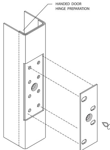
Hinge size and thickness is determined from the hardware schedule. On the hardware schedule, each door opening is listed which identifies the usage of specific hardware. This information is available on every opening on a job. By checking the hardware schedule against each door on the job, it can be determined what hardware preparations are required, such as:
