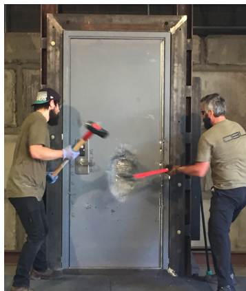
Image from actual forced entry testing
